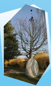
**The Sonopode®** is a specific equipment that has been developed by Bruitparif to make the installation of a noise measurement station easier, particularly in the case of air noise nuisances where the expert stations used require a solidly anchored mast. It requires no connection thanks to:
